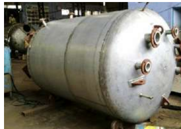
MS Storage Tank
